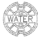
VALVE BOX LID CAST IRON, TWO PIECE, SLIP TYPE
