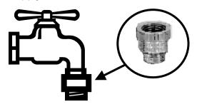
Another way to prevent backflow with a garden hose is to use a device known as a vacuum breaker. Vacuum breakers are available at hardware and home improvement stores. They are simple, inexpensive, and screw right onto your outside faucet to prevent contaminants from being siphoned back into your plumbing and the public water system.
